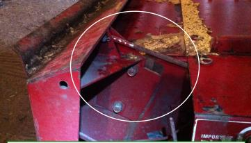
On International combines, check the pitch of the header on the feeder house. To do this: loosen the nuts and adjust the rod forward so that the feeder house angles forward and cutter bar lowers.
