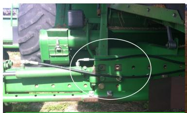
On John Deere combines (i.e. 9600), check the position of the back axle. Adjusting from the upper to lower position can allow the cutter bar to cut 2-3" lower.
